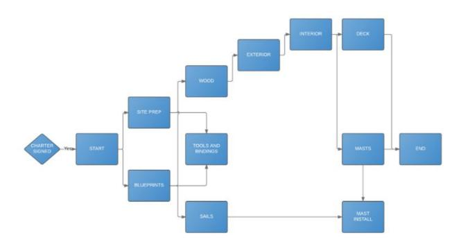
The network diagram typically moves from the left to the right (START to END) and includes forks or branches along the way. For example, on the lower right of the diagram, the MAST INSTALL action has a dependency on MASTS and SAILS. Literally speaking, we cannot install the mast in the ship without sails and the mast first being built.
